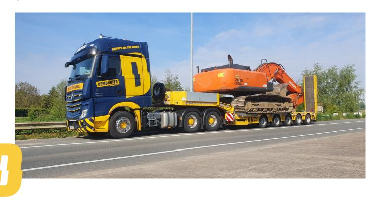
Semi low-loader combination for heavy-duty work. This low loader combination can transport machines, loads up to 50 T.
